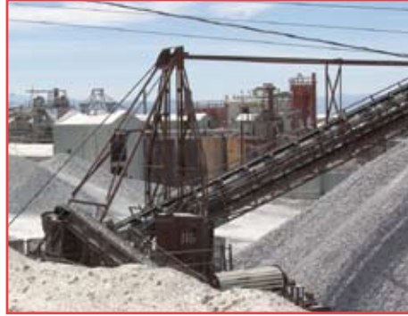
The on-site plant crushes, processes, and blends the mined ore creating over 40 specialized products.
