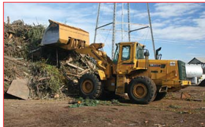
Compost is a 24/7 activity and a Kawasaki 80ZV-2 equipped with a 7.25-cubic-yard Tink roll-out bucket helps move the job along at a rapid pace.
