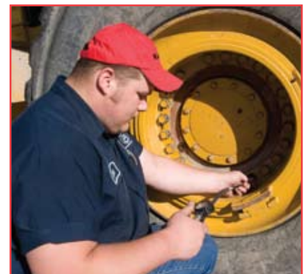
Check tire condition and air pressure.
