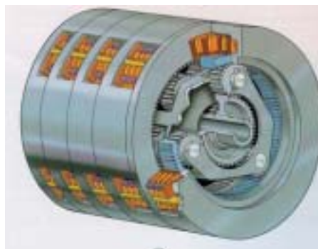
Inside transmission with planetary gears
